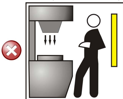
Fig 9 - Wrong light curtain positioning
