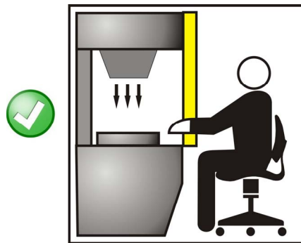
Fig 8 - Correct light curtain positioning
